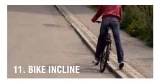
The bike incline will connect Penn Avenue to Garfield hilltop park. A bike incline lifts cyclists, astride their bicycle, up a hill at three to four mph. The lift runs along the curbs: riders leave one foot on a pedal and the other on a foot plate that moves smoothly up the hill. Users buy keycards, just like subway cards. Only two such bike inclines exist. The first and original lift is in Trondheim, Norway, a city of only 173,000 people. The second is in Brussels.
